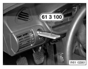
Press together retaining clips with special tool 61 3 100 and slide backwards to remove.
