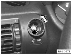
Unfasten lock nut and twist button to remove.
