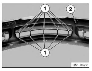
Unfasten retaining washers and remove air grill. Lift cover (2) off towing eye and unfasten catch band.
