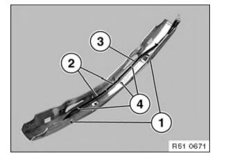
Version with headlight cleaning system: If necessary, unfasten expanding rivets (1) and screws (2). Remove support member (3) with hoses, replace faulty cable ties (4) if necessary.
