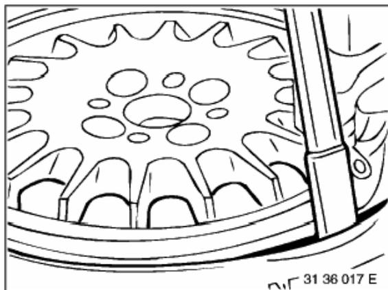
Swing or fold mounting pillar into position and let it engage.
