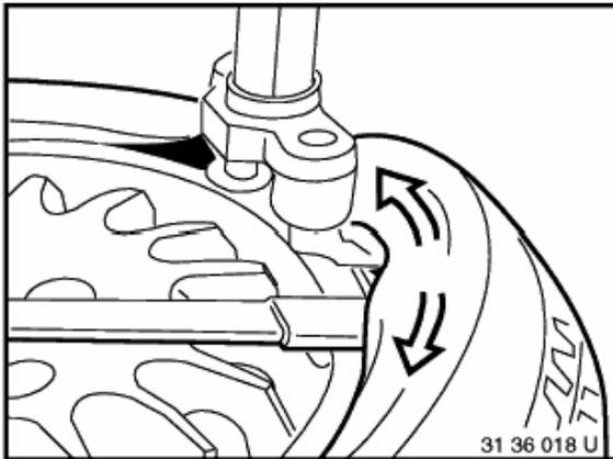
Let mounting machine run back a short distance (counterclockwise) so that tire bead can slide fully onto mounting finger.
