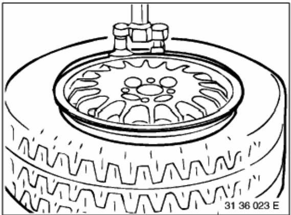
After mounting, first release clamps and then inflate tire (without valve).
