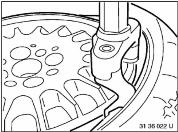
Turn wheel again into fitting position so that valve is 180° opposite mounting head.
