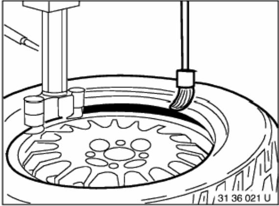
Swing or tilt mounting pillar into position and lock.
