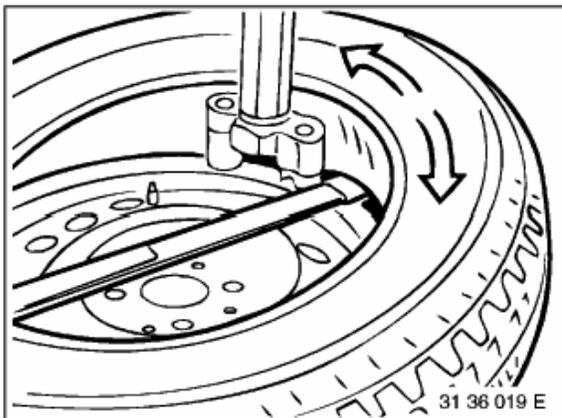
If the upper bead is pulled off the rim, also lift the bottom bead over the mounting finger with the tire iron.
