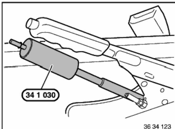
Unscrew locknut using special tool 34 1 030 and loosen cable completely.
